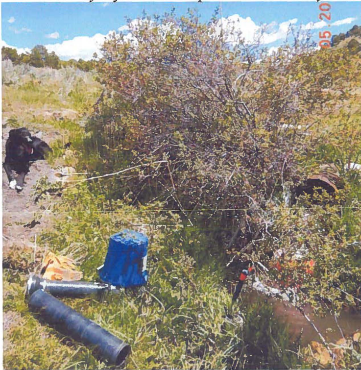
Photos 7a-b – a)(upper photo) Four-Eyed Nick’s springbrook with 4” screened intake for buried irrigation pipeline in lower center of photo (below orange flagging), looking ENE; flow of 112 gpm was measured from 16” steel pipe discharge on right behind brush, for entire flow of springbrook and comingled sources; site is at an elevation of 6590 ft, ~1,000 ft WSW of 4ENS proper; b)(lower photo) V03657 upper claimed sub-irrigated POU, looking ENE with Diamond Peak on skyline; 4ENS proper is out of view ~75 yards behind photo location; several of the other undeveloped spring sources are in upper portion of meadow in middle distance; porta potty for scale.
