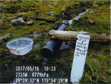
Upper Photo: Spanish Gulch Spring flow measurement site, looking south, with fenced spring source to left of ATV; Lower Photo: closeup of site with measured flow of 2.8 gpm (excellent).
