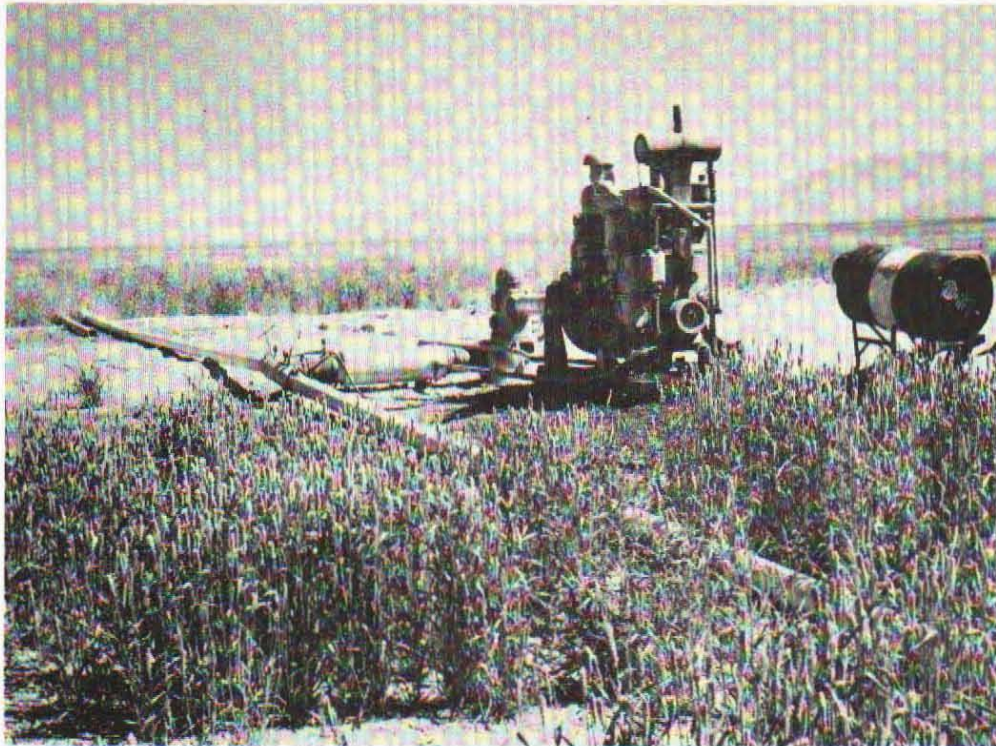
Photograph 5. View northwest showing typical well installation in Diamond Valley in field of small grain. Discharge from well goes directly into aluminum pipe which, in turn, is connected with sprinkler lines.
