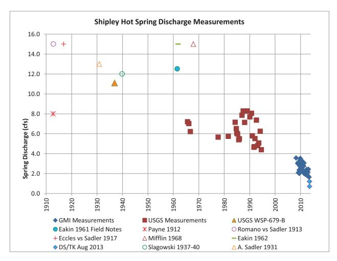
Figure 1 – Shipley Hot Spring Discharge Measurements and Reported Discharge, 1912 to 2013
