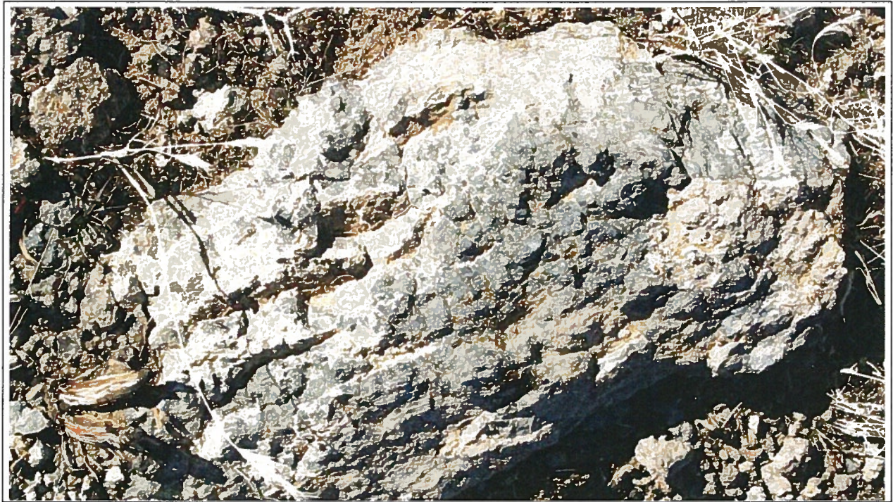
FIGURE 7 SAMPLE OF DELAMAR LAKE TUFF, SHOWING PUMICE FRAGMENTS AND LITHOPHYSAE FROM NEARBY OUTCROP EAST OF MONITOR WELL 182W906M
