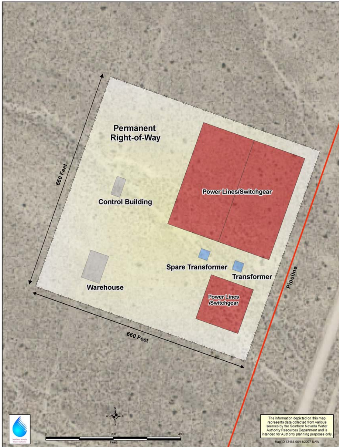
Figure 2-23 Preliminary Primary Electrical Substation Site Plan
