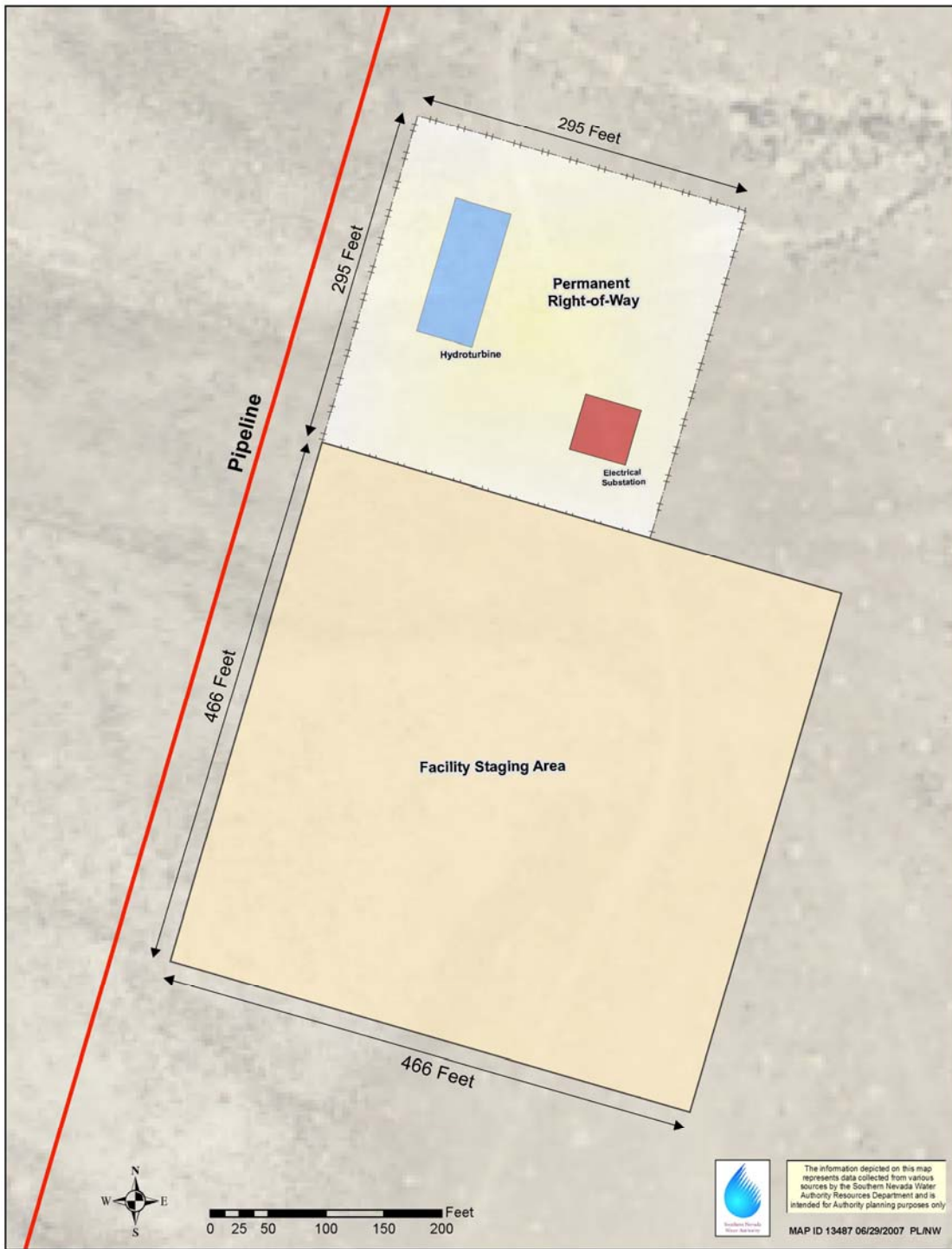
Figure 2-24 Preliminary Hydroturbine Energy Recovery Facility Site Plan
