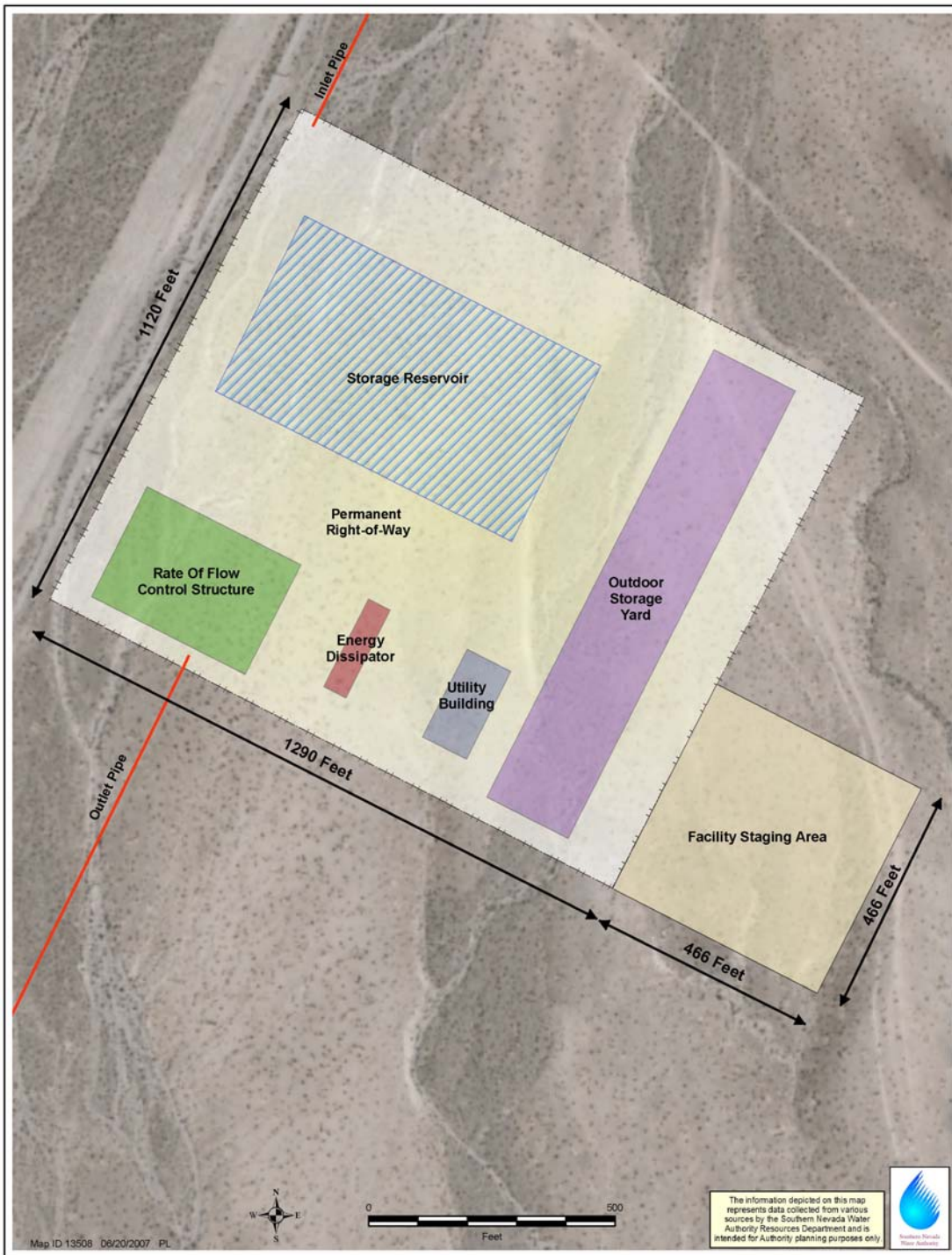
Figure 2-18 Preliminary Buried Storage Reservoir Site Plan
