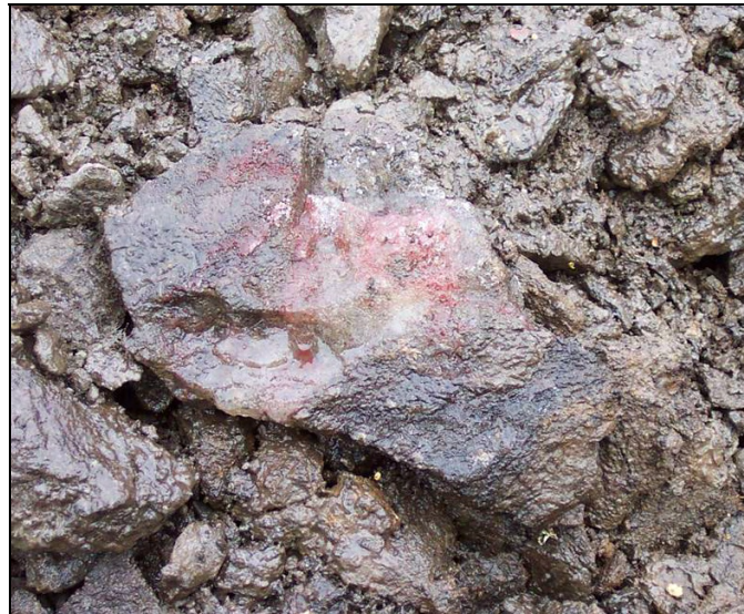
Figure 40. When alpha, alpha-dipyridyl dye is applied to a soil containing reduced iron, a positive reaction is indicated by a pink or red coloration to the treated area.
