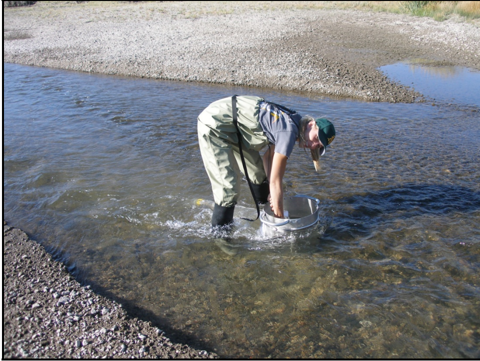
Figure 2.2-12. Depiction of Hess sampler being used at invertebrate site 5.
