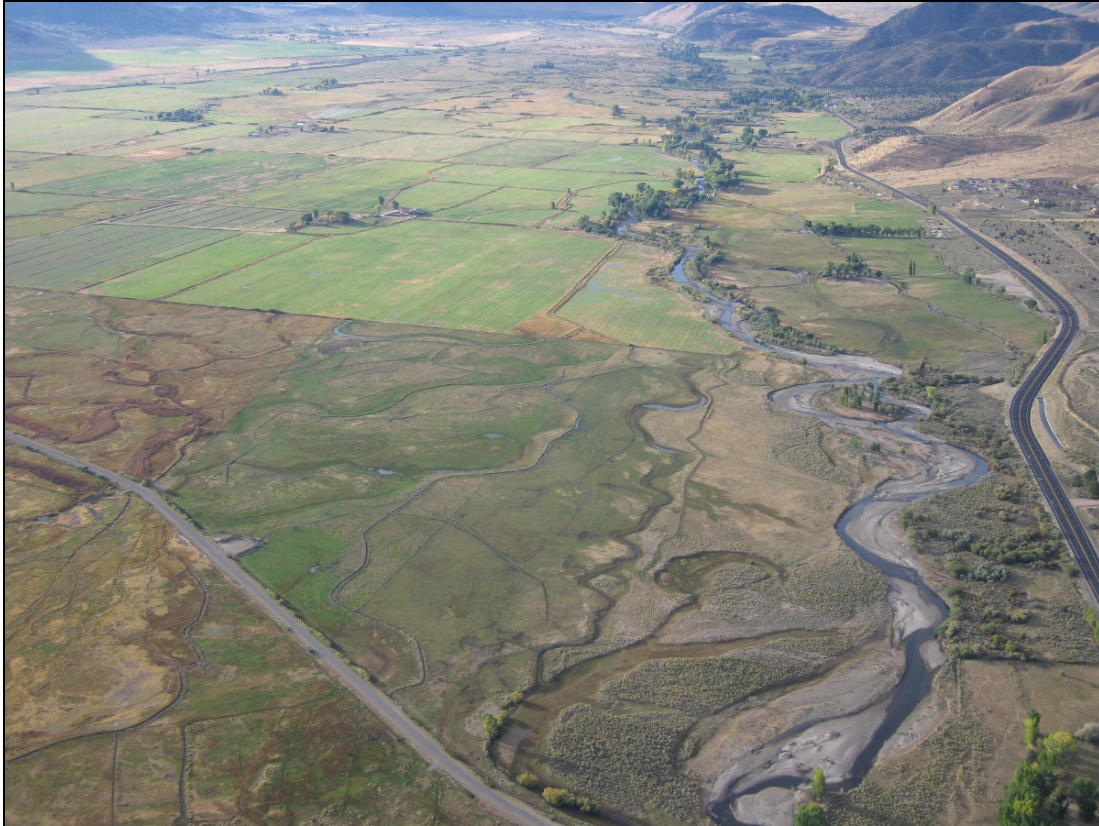
Figure 2.1-38. Low elevation oblique aerial photo of the West Walker River in WW4 in the Antelope Valley. The view is looking upstream. Note the geomorphic features in the foreground such as channel scars on the floodplain, and the large point bars in the active channel.
