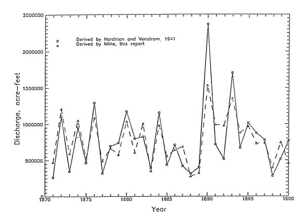
Figure 12.--Comparison of estimated pristine discharges for the Truckee River (after Hardman and Venstrom, 1941).
