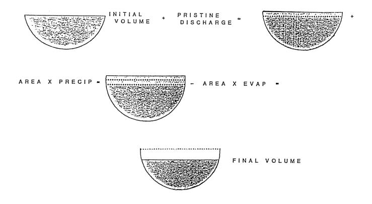
Figure 4.--Schematic diagram showing method of calculating changes in lake level.
