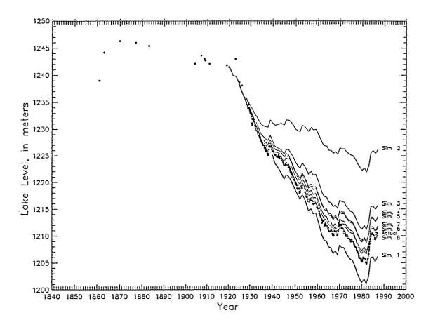
Figure 7.--Model-calibration results for Walker Lake (refer to Table 5 for summary of model input data).
