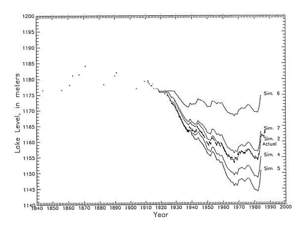
Figure 15.--Model-calibration results for Pyramid Lake (refer to Table 7 for summary of model input data).
