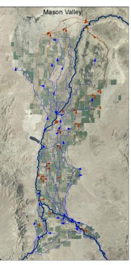
Ditches and drains of lower Mason Valley with flow directions.
