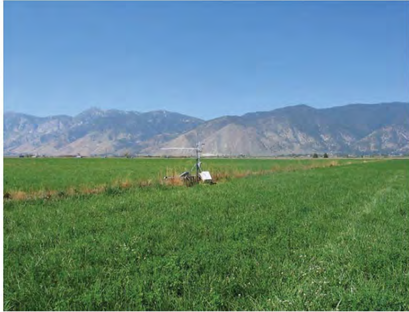
Figure AP7. USGS Bowen Ratio micrometeorological weather station located in a field of irrigated alfalfa (modified from Maurer et al., 2005).
