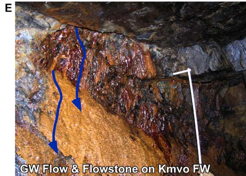
Figure 18.—Continued Photographs of the Standard fault vein from Levels 3 and 5 in the Standard Mine. (D) Asymmetric groundwater flow on the Ohio Creek footwall principal slip surface of the Standard fault vein in Level 5. Note the Wasatch hanging wall is nearly dry. (E) Detail view of groundwater flowing (blue arrows) on the tripe-like (orange-beige to ochre) and drapestone-like (blood-red) flowstone types on the Ohio Creek footwall principal slip surface of the Standard fault vein in Level 3. CRG, clay-rich gouge; HW, hanging wall; HWDZ, hanging wall damage zone; FW, footwall; FWDZ, footwall damage zone; GW, groundwater.
