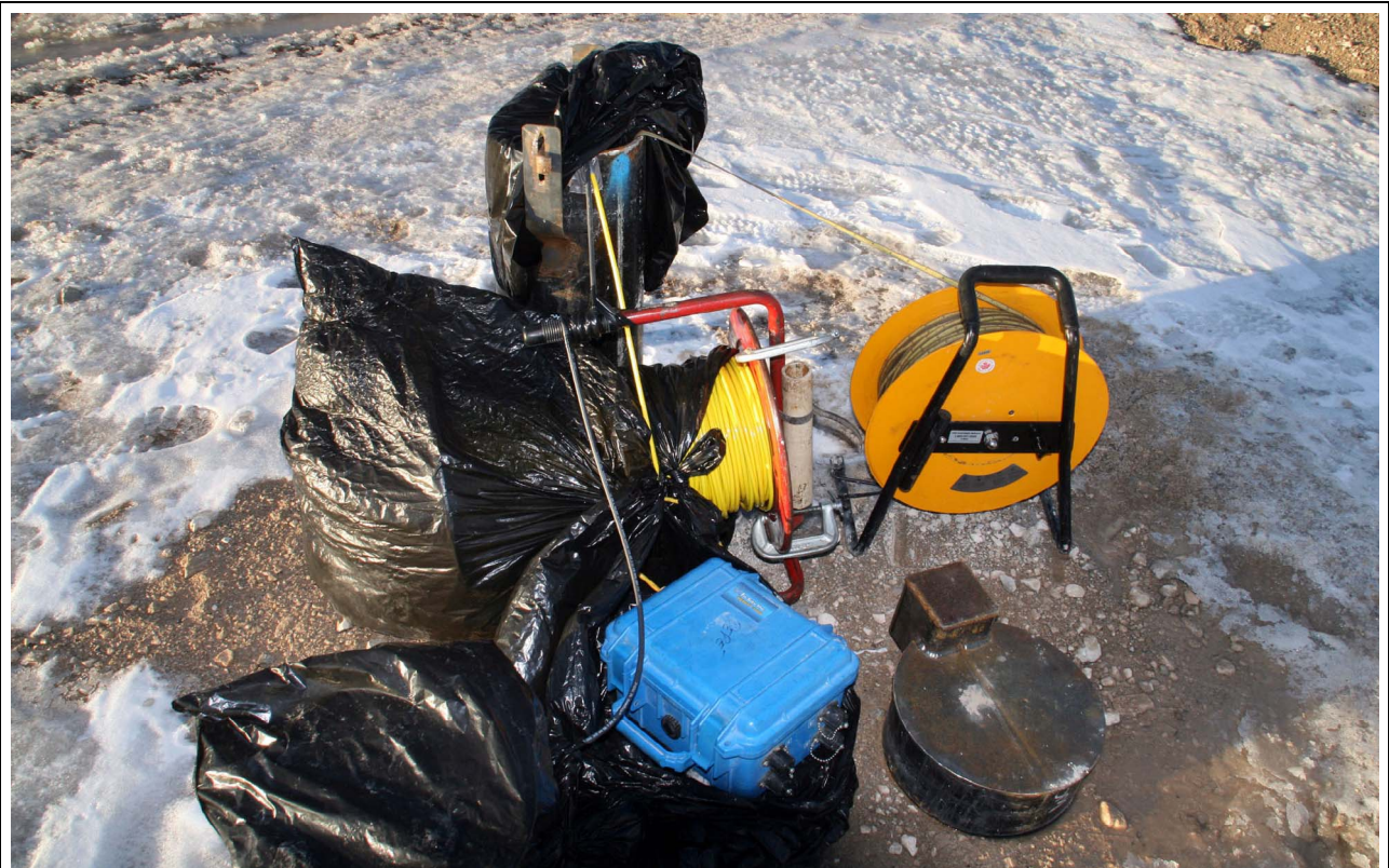
Figure A-5 Monitor Well SPR7007M with Water Level Measurement Instrumentation
