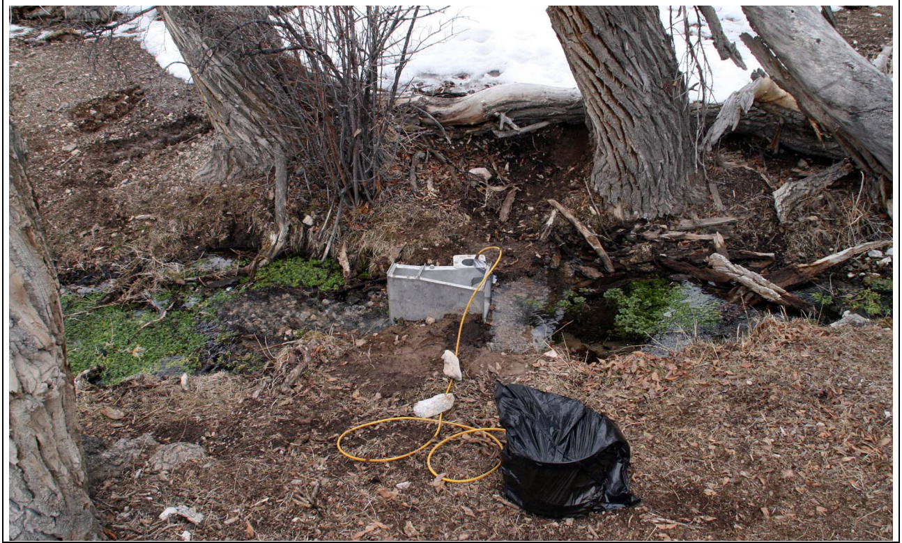
Figure A-6 North Swallow Springs Flume and Temporary Transducer
