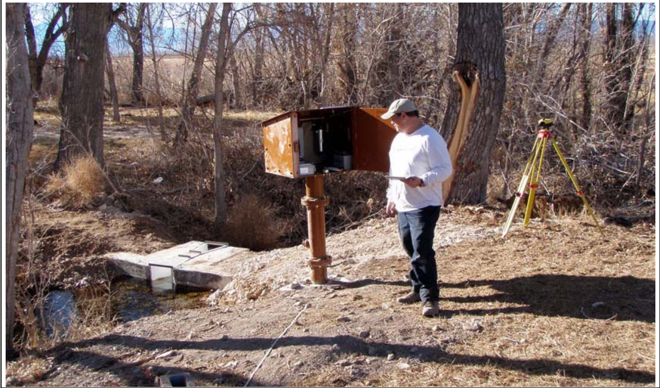
Figure E-1 Flag Spring 2 Flume and Continuous-Recording Instrumentation, Fall 2009
