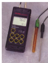
Figure D.3: pH and ORP meter with thermistor thermometer
