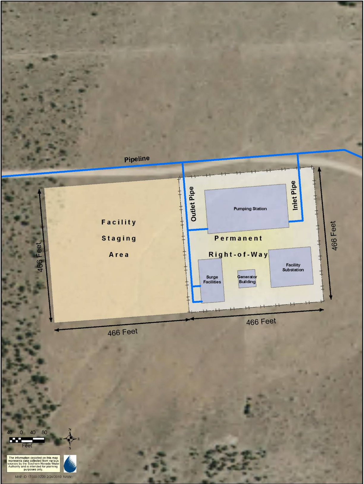
Figure 2-16 Preliminary Lake Valley Pumping Station Site Plan
