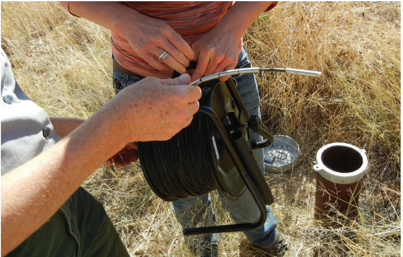
Comprehensive and consistent monitoring and measurement is the cornerstone of adaptive management. The device shown here is used to measure depth-to-groundwater.
