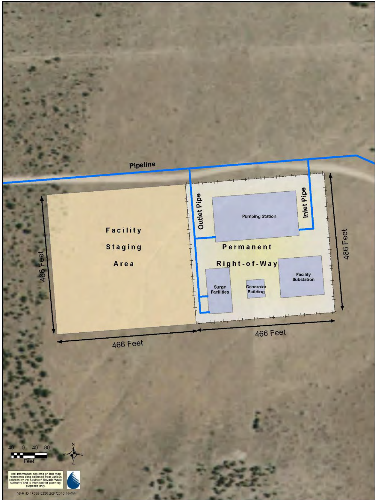
Figure 2-14 Preliminary Lake Valley Pumping Station Site Plan
