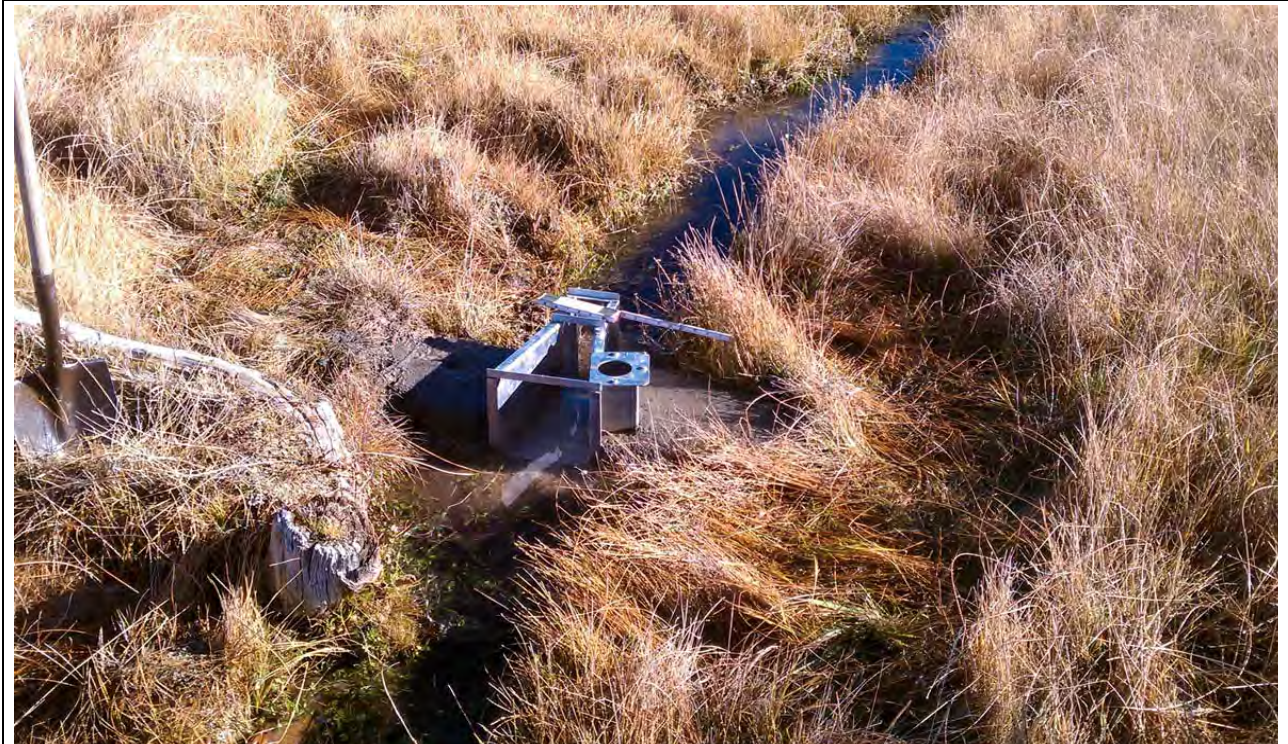
Figure 16-5 Flume Installation at Cleveland Ranch Spring North
