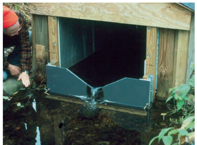
Surface-water outflow from Mirror Lake was measured with a combined weir and flume.
