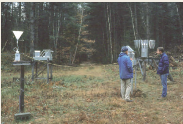
Multiple gages reduce the inaccuracy of precipitation estimates.
