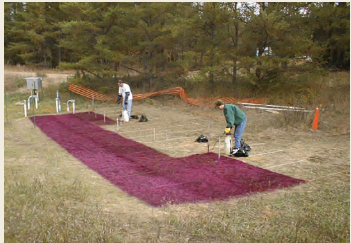
Applying dye tracer to land surface at research site in Minnesota.
