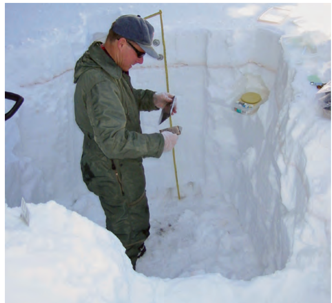
Snowpits are dug to determine water content and chemistry of snowpacks.
