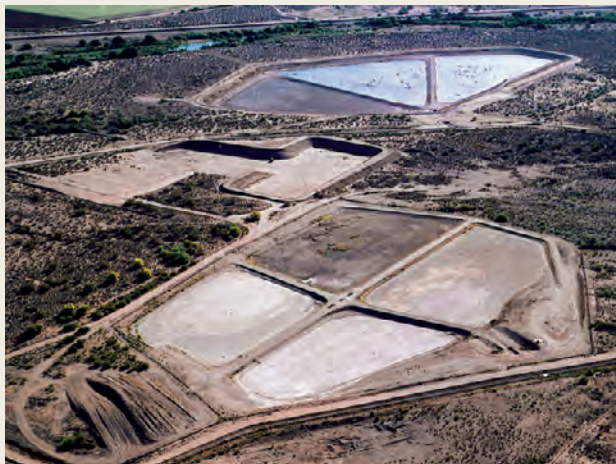
Natural recharge to aquifers can be augmented by induced recharge through spreading basins such as these in the Avra Valley of Arizona.
