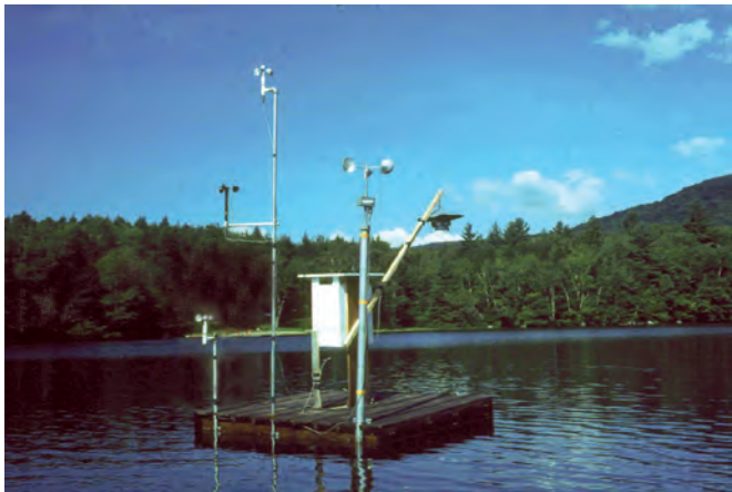
Instrumentation to measure evaporation from a lake.
