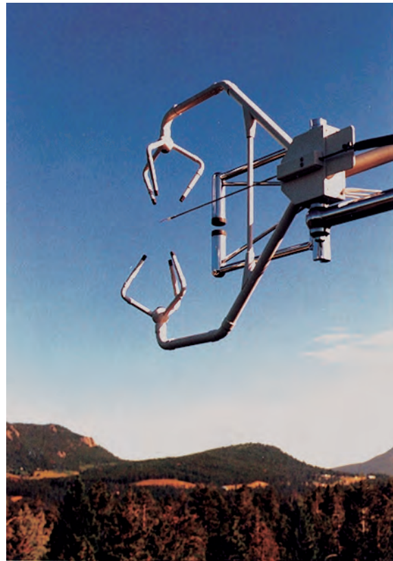
Instruments used in eddy correlation measurements of evapotranspiration.
