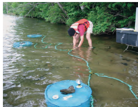
Seepage meters are used to measure the exchange of water between surface water and the subsurface.
