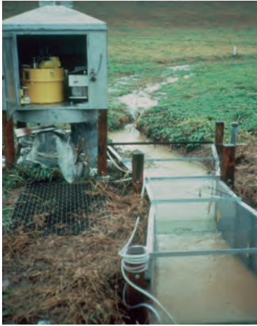
Flumes and weirs were used to measure runoff.
