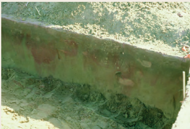
Dye tracer is visible in trench excavated beneath application area.
