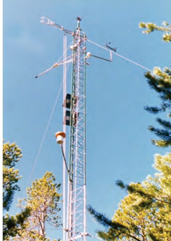
Tower to measure evapotranspiration in a forest.
