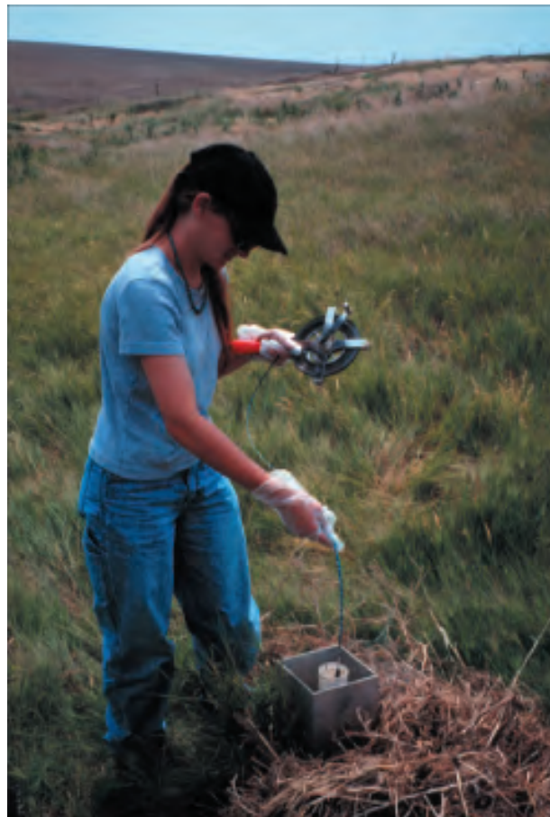
Measuring water levels in an observation well in Colorado.
