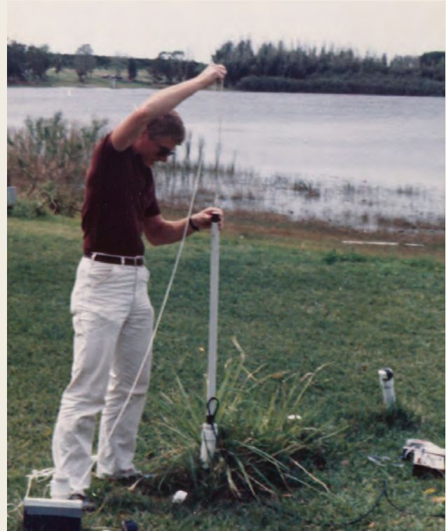
Performing slug tests to determine aquifer hydraulic conductivity.
