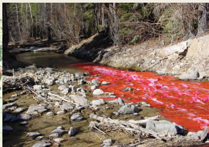
Tracers are used in streams to measure traveltimes.
