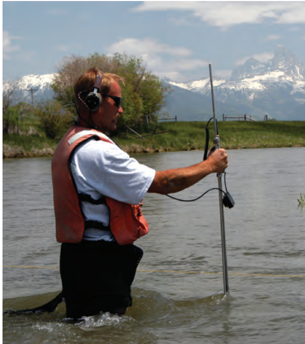
Discharge is determined with measurements of stream depth and velocity.
