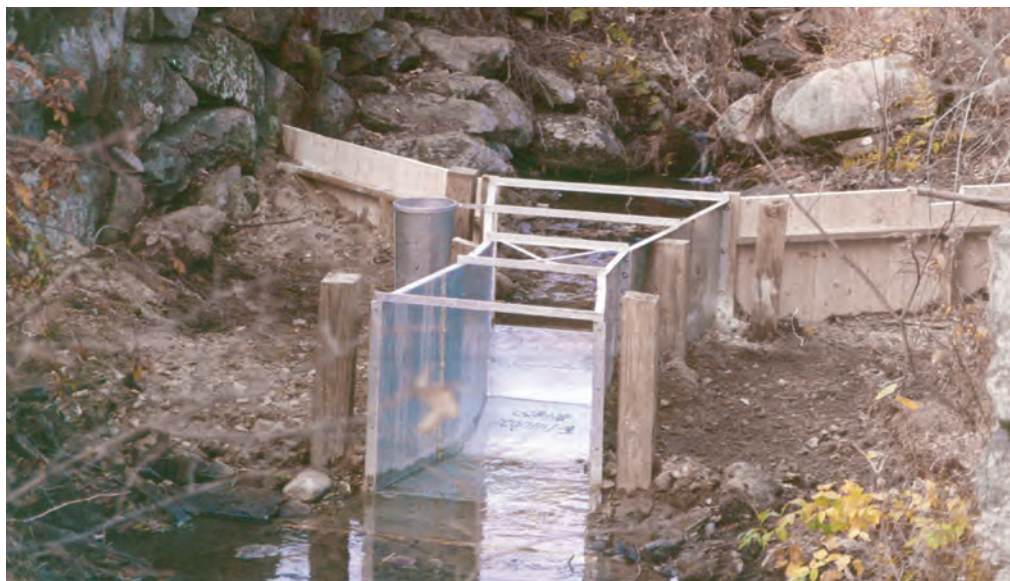
Flumes can be used to measure discharge in small streams.
