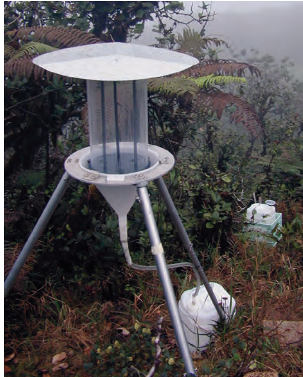
Fog drip collector in Hawaii. In some areas, fog drip is the primary form of precipitation.
