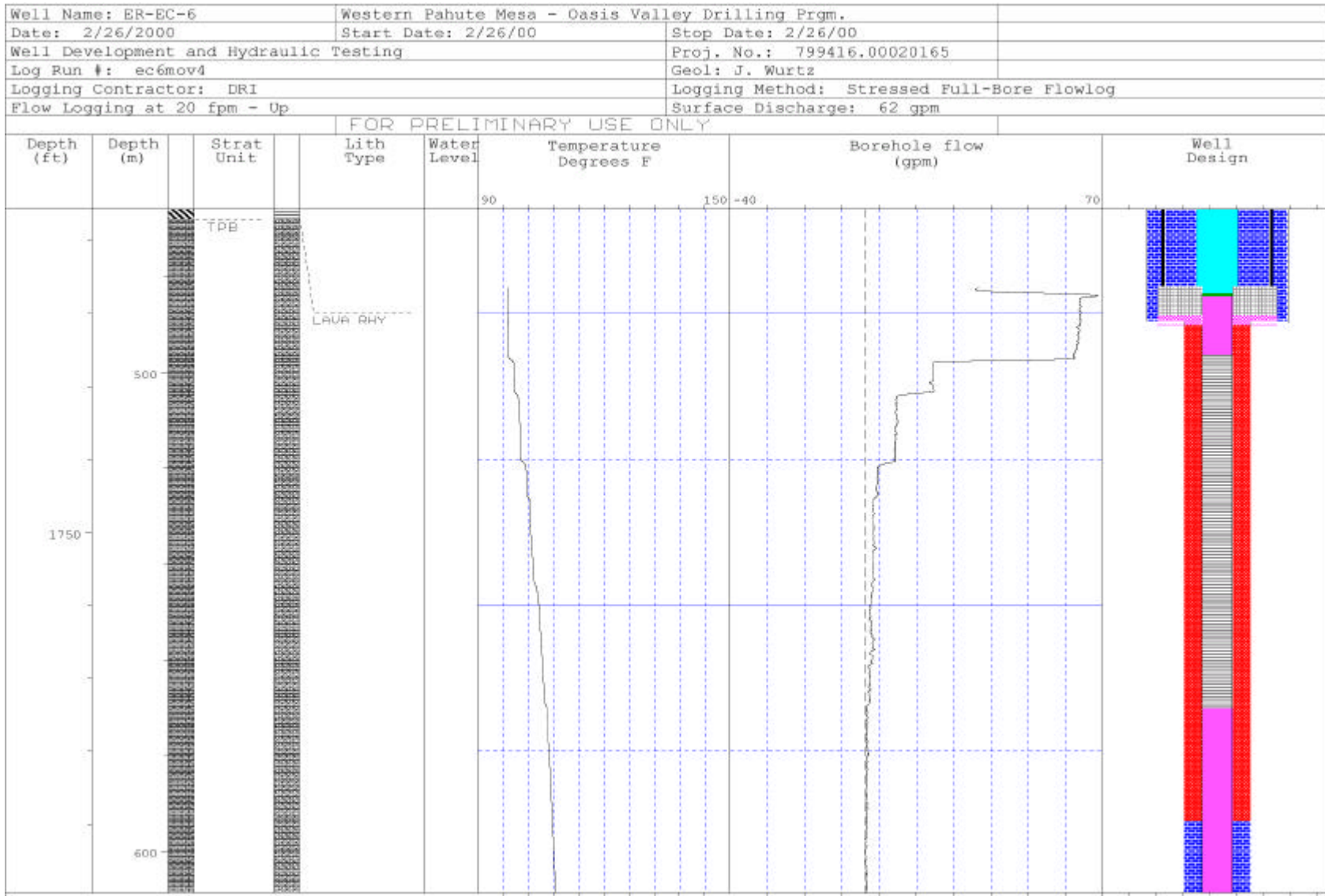
Figure A.3-8 Flow and Temperature Log for the Upper Interval at 62 gpm
