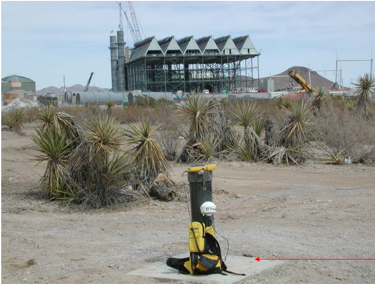
Preparing to set up a GPS data gathering station on Well GV-PW-MW1 in Garnet Valley
