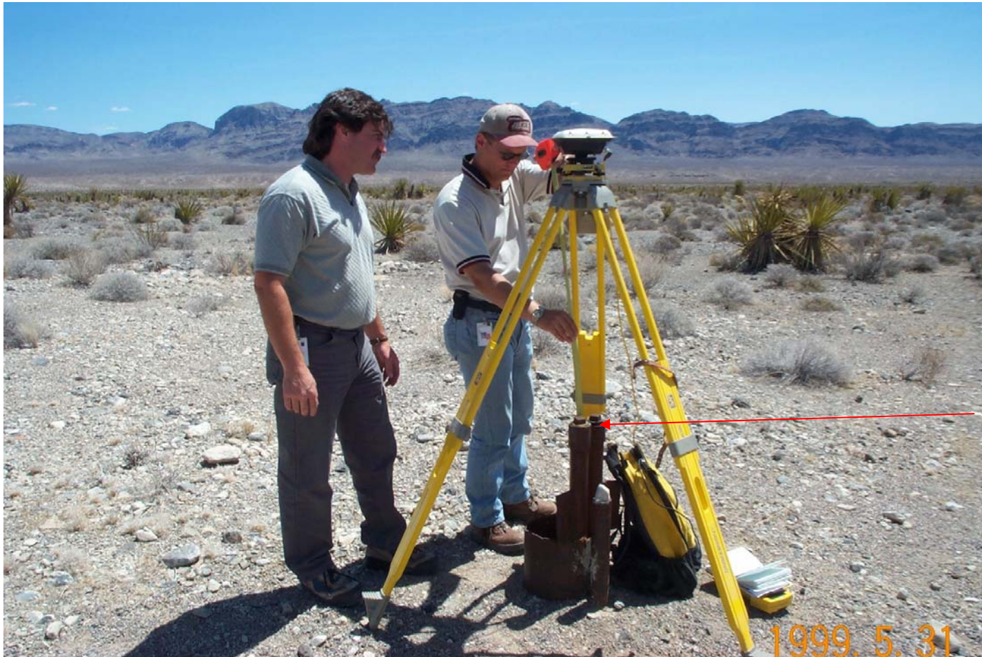
Survey team setting up a GPS station on Well CE-VF-1 in Coyote Spring Valley (date on picture is an error)
