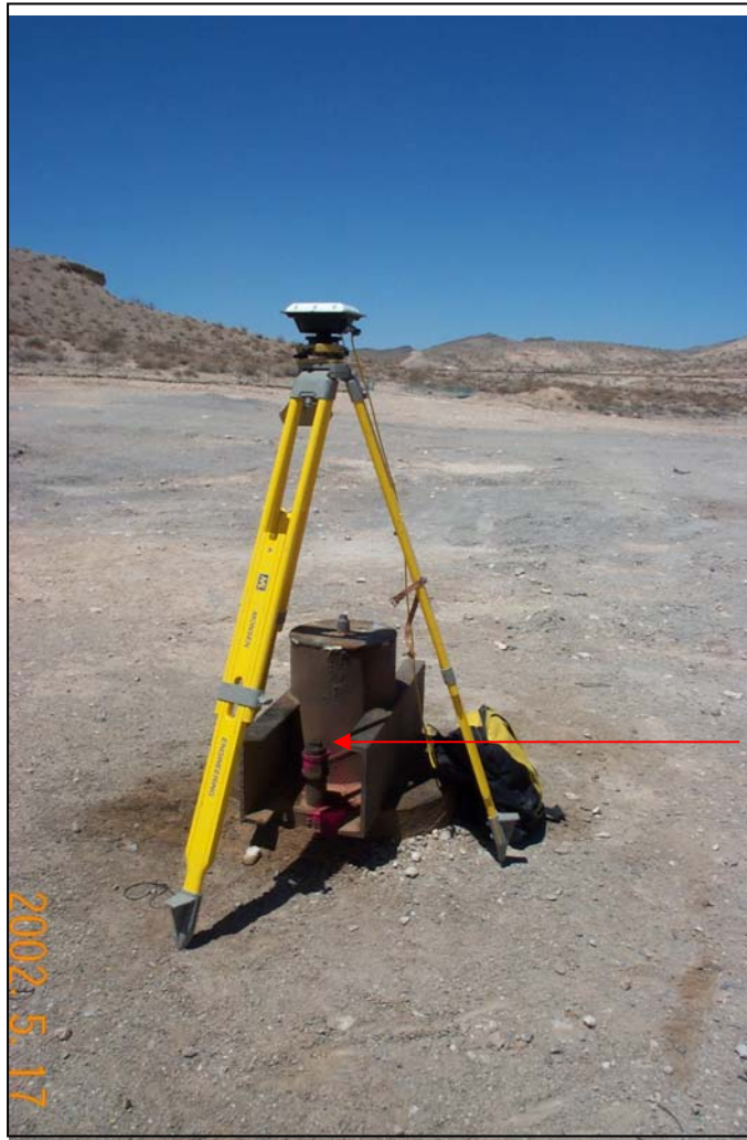
GPS setup at BM-DL-1 (Apex-1) in the Black Mountains Area (Well has since been fenced)
