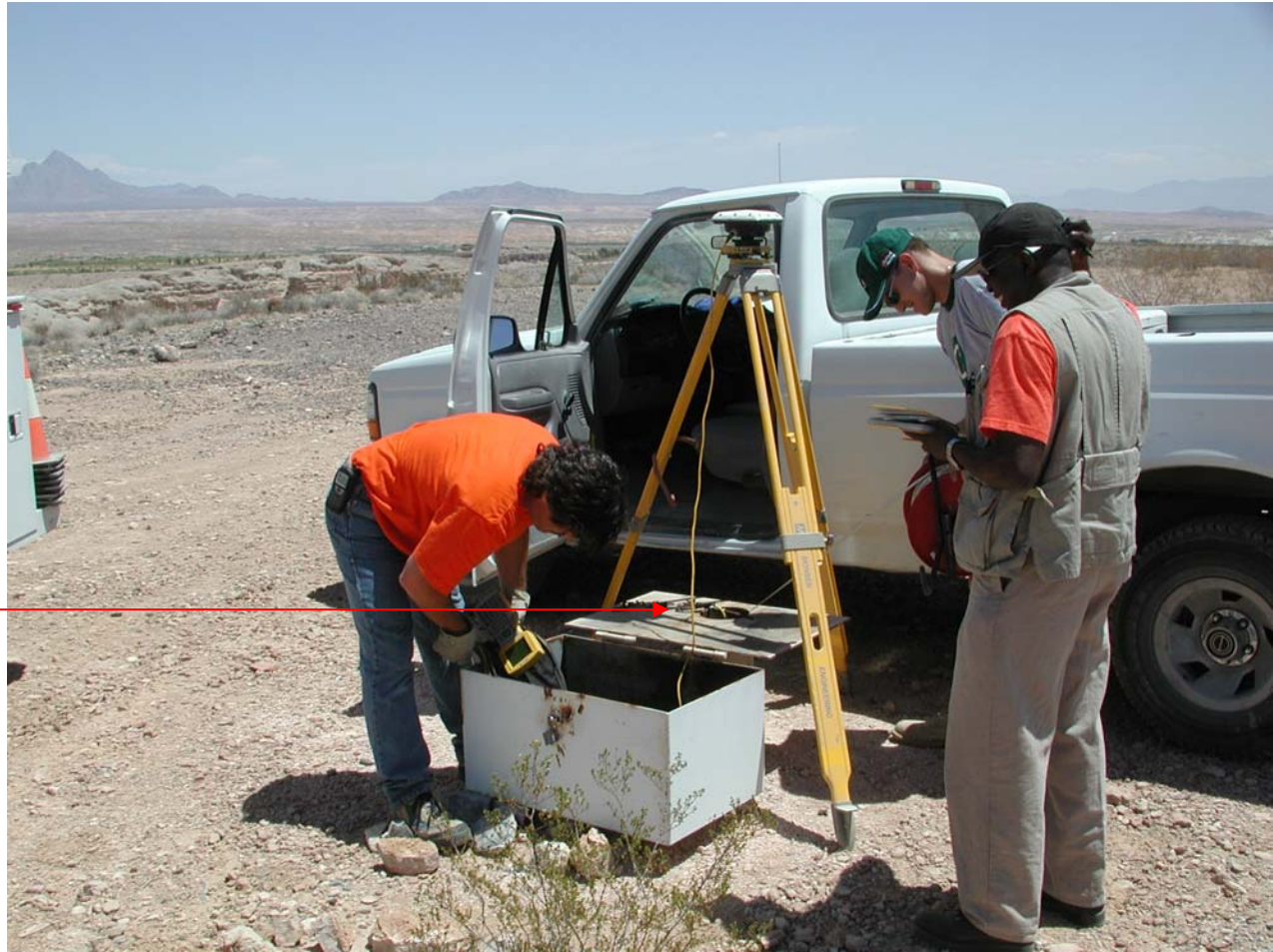
Survey team setting up GPS data gathering station on Well EH-4 in the Muddy River Springs Area
