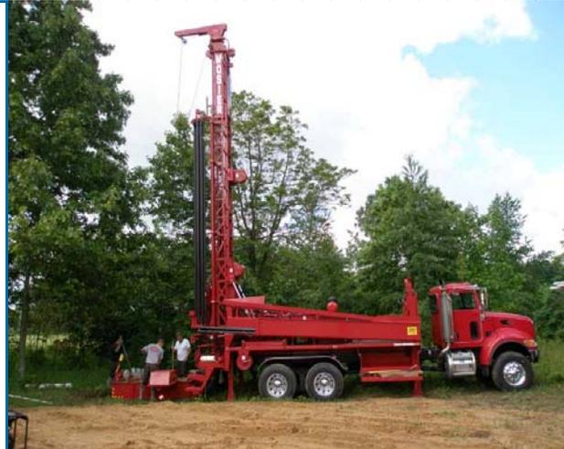
Schramm T450MIIA, top head drive, air rotary, mud rotary and DTH hammer drilling methods.
